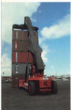
A ContChamp can stack up to five high in the first row.
