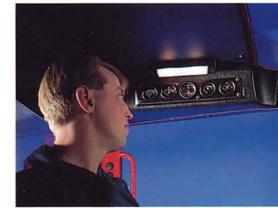
The instrument panel is placed to the left in the cab and offers the driver an immediate indication of all main operational functions.
