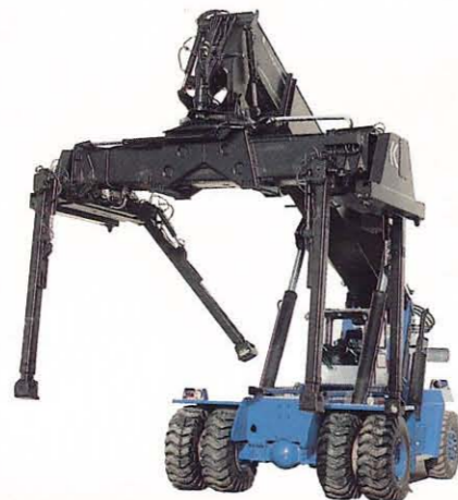
The attachment, equipped with two sets of retractable trailer handling legs, is electro-hydraulically operated from the cab.
