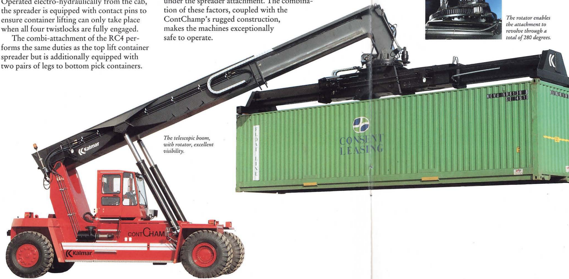
A set of lights on the boom indicate when all twistlocks are locked and only then can lifting operations take place.
