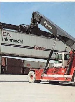
Flexibility, large outreach and lifting capacity characterises the ContChamp.
