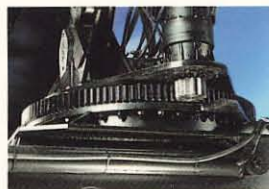
The rotator enables the attachment to revolve through a total of 280 degrees.
