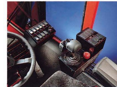
The hydraulic controls, steering wheel and driver's seat are individually adjustable.
