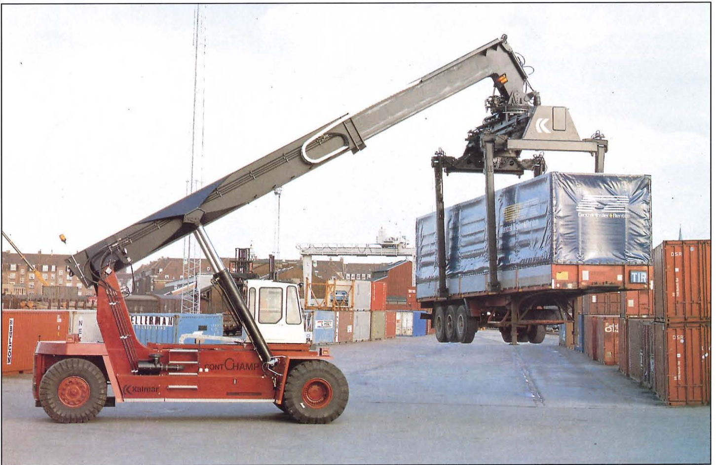
The boom has its own distinctive, high strength steel design, and it can be operated by a double-action protrusion cylinder.
