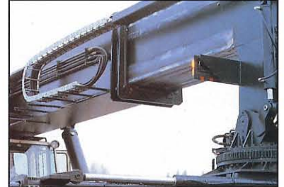
Hoses and cables run in a guide chain to reduce the risk of damage.
