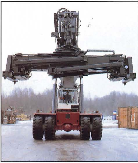
The Combi unit is designed for handling trailers and 20'-40' containers, and is operated by electrohydraulic means from the driver cockpit.
