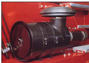
The intake air is purified in a two-stage air cleaner. In the first stage, coarse particulates are separated by a 'cyclone' effect and collected in a dust container. Stage two is performed in a 'main cartridge'. There is a safety cartridge on the inside of the main cartridge which protects the engine from air pollution if, for example, the main cartridge becomes damaged.
