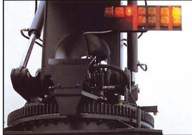
To help the driver, the machine is fitted with an indication panel that is easy to read and which indicates the functions engaged.
