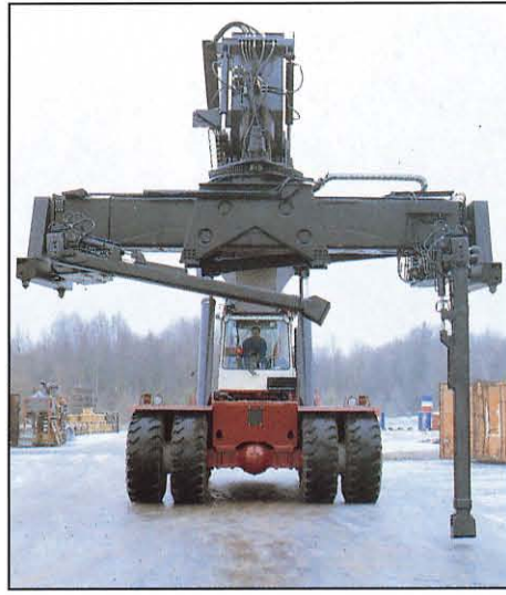
The Combi unit is designed for handling trailers and 20'-40' containers, and is operated by electrohydraulic means from the driver cockpit.
