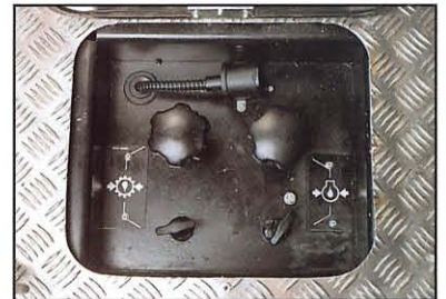
Checking the oil level and topping up are performed in special service covers.
