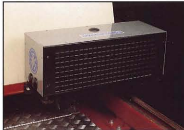
The in-cab climate unit maintains a pleasant working climate inside the cab. The unit is operated by switches on the instrument panel and a control below the panel.
